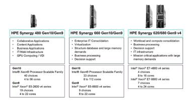
Figure 6-5: Compute module workload comparison.
