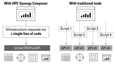
Figure 4-5: Unified API enables infrastructure requests using a single line of code.
